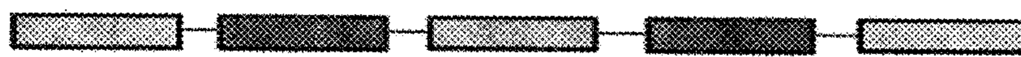
multiphase block copolymer (A,B: oligomers)
