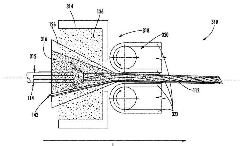
core elements. Further, the binder film loads the core elements normally to the central strength member such that contact between the core elements and central strength member provides coupling there between, limiting axial migration of the core elements relative to the central strength member.
