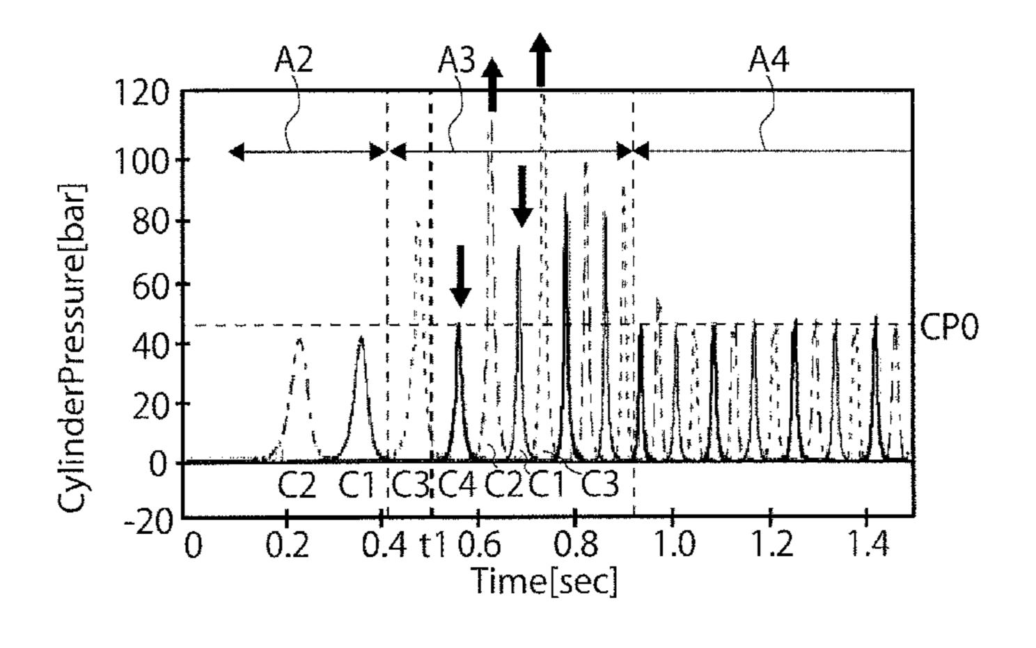
device for controlling injectors such that fuel injection amounts of respective cylinders become uneven when the rotational speed is within the resonance-rotational-speed region.
