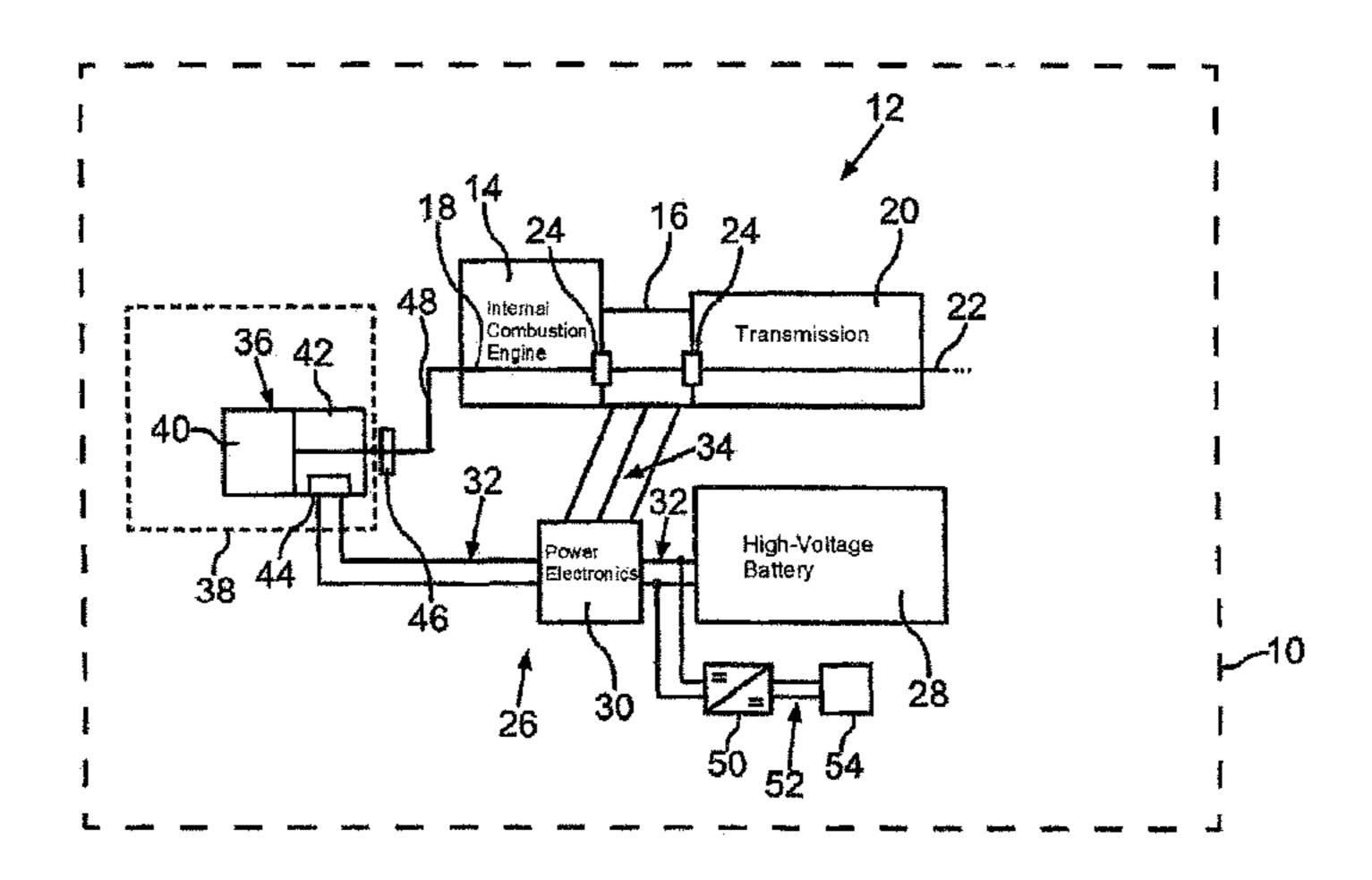
couples the electric motor of the air conditioning system with the internal combustion engine in response to a control signal.
