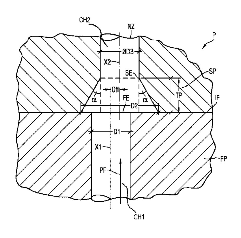
a first tapered portion (TP) which narrows in the second portion (SP) at increasing distance from the interface (IF).
