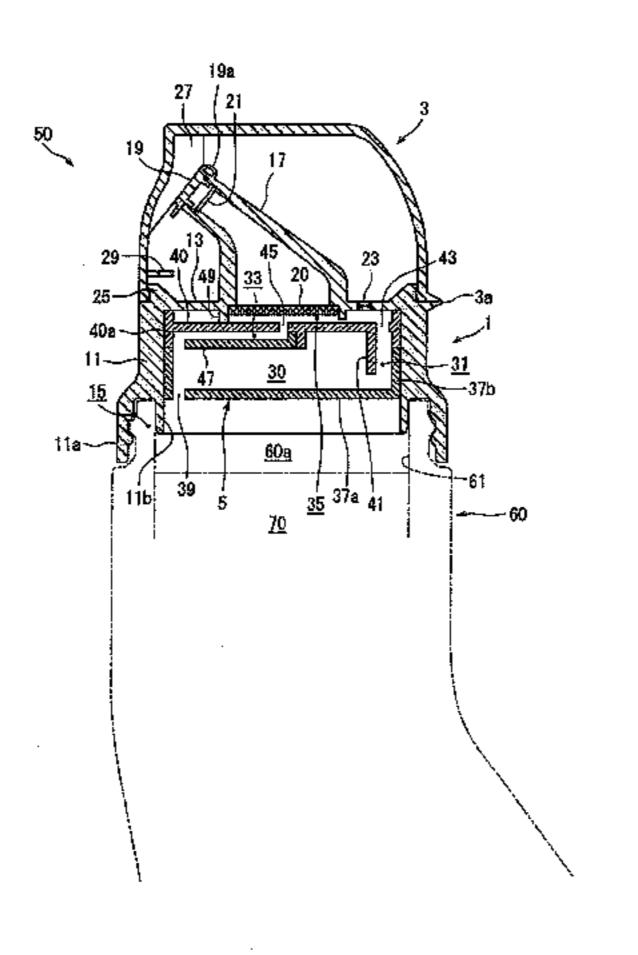
pipe defines an air-liquid mixture flow path. When the squeeze container is tilted and squeezed, the content liquid is ejected in a foamy state from the leading end of the ejection pipe.
