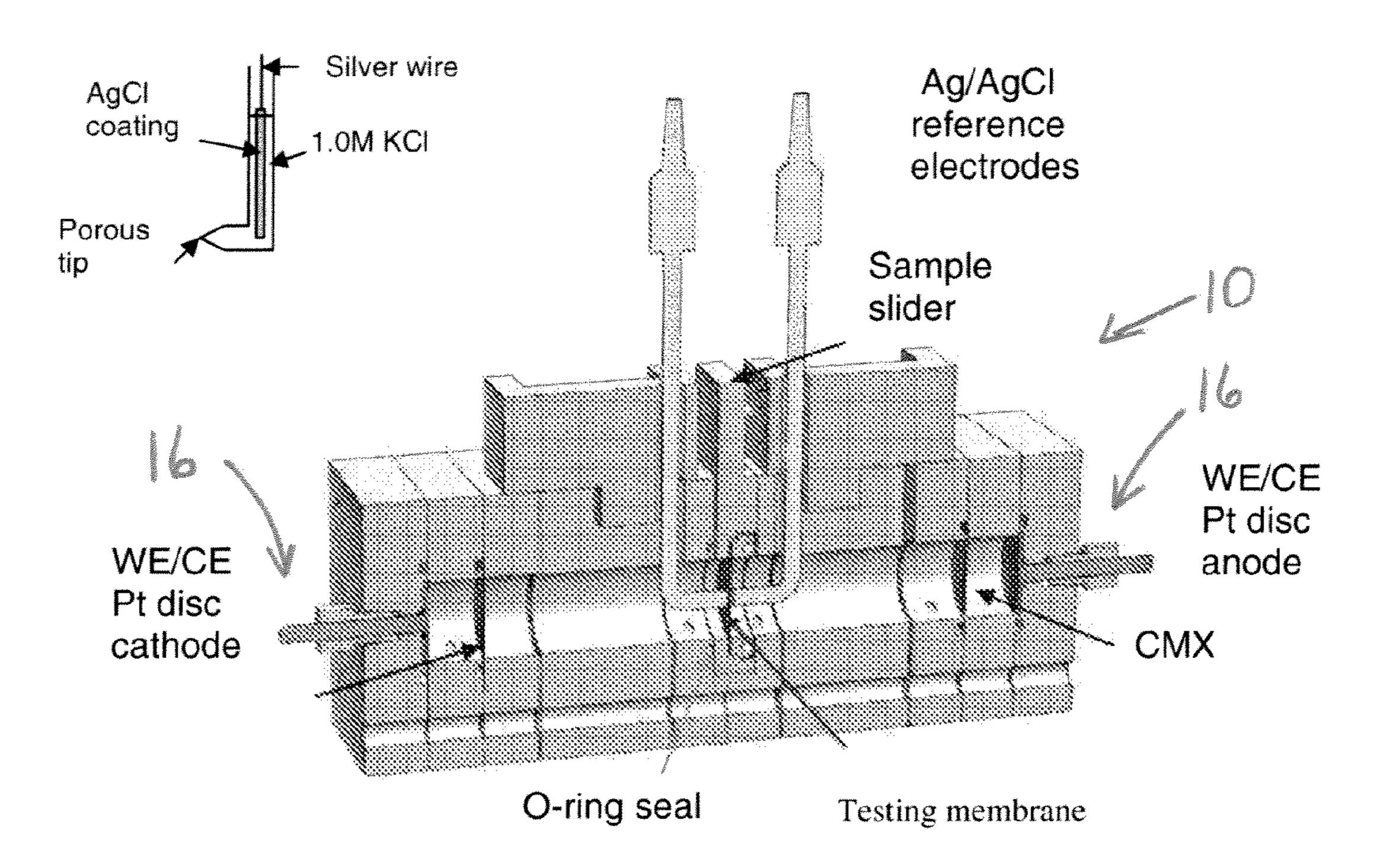
Construction of the membrane test cell and the reference electrode
