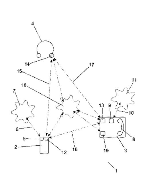
determine a relationship between the first call announcement signal (21, 41) and the first user accept signal (23, 31), and to cause the desktop telephone system (1, 51, 61) to establish an audio connection (15, 16, 17, 44, 47, 48) between the first gateway device (2, 3, 62, 63) and the first sound interface device (2, 3, 4, 8, 62, 63, 64) in dependence on the determined relationship.
