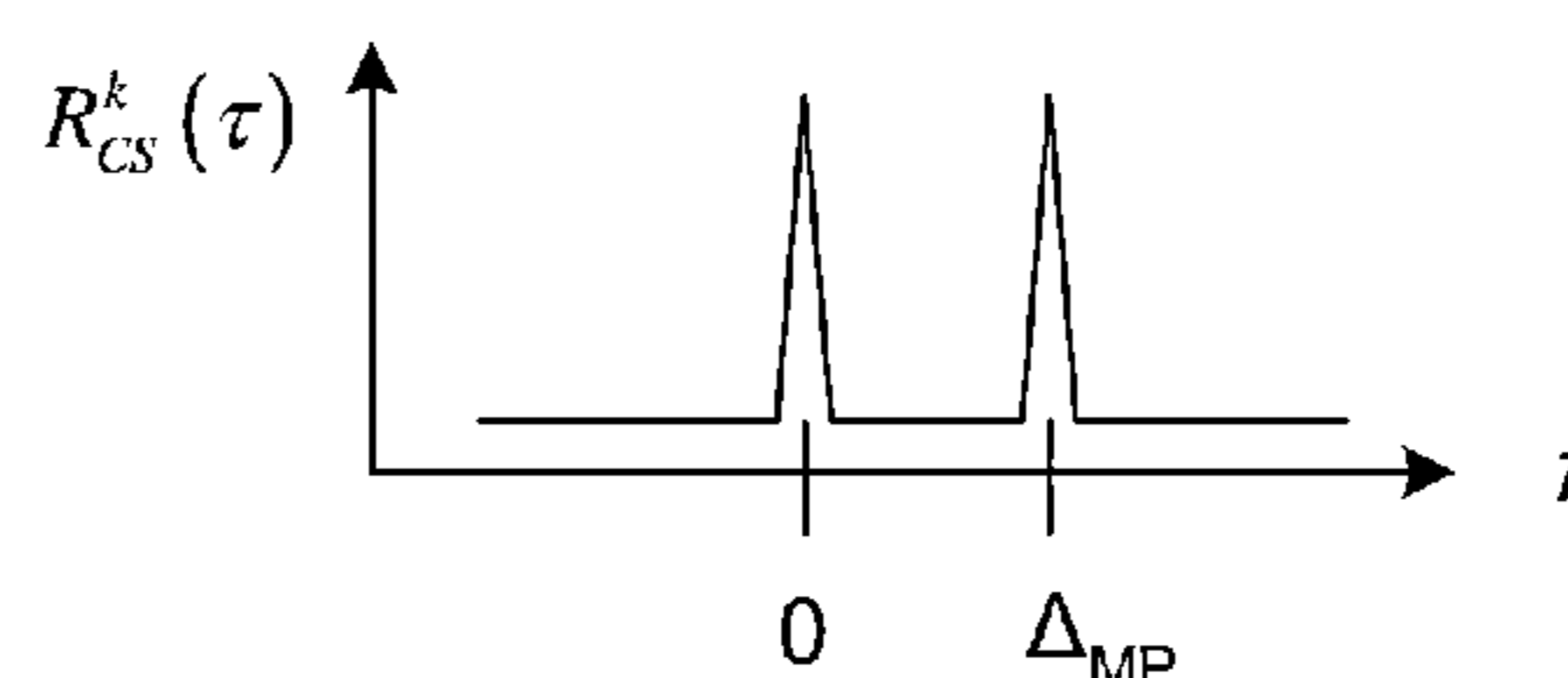
Cyclic shift-based autocorrelation of (two-path) multipath signal y(t)
