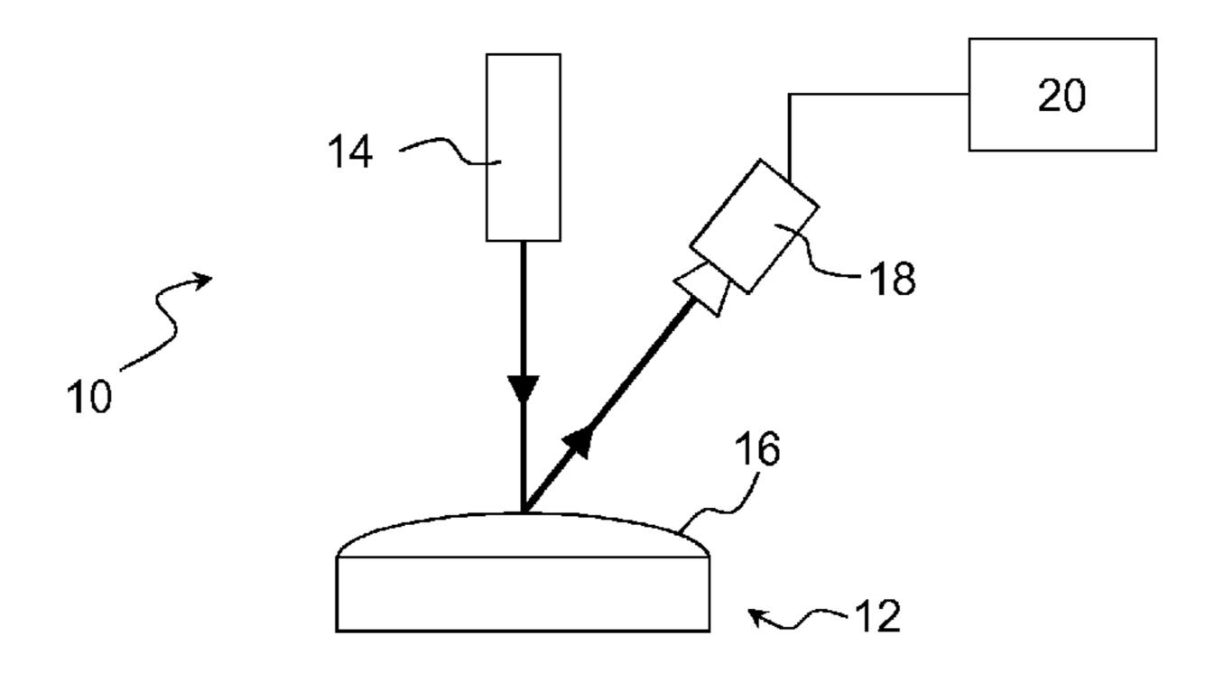
at the emission wavelength by the illuminated surface is collected to build an image of the surface, and the surface image is processed to apply metrics to compare the image with reference data specific to the given geometrical feature.
