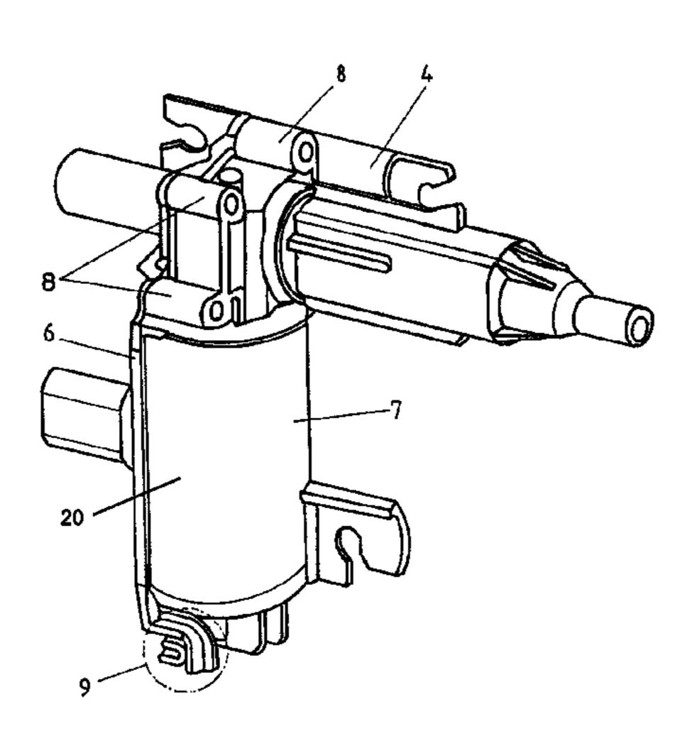
large peripheral edge of the connecting part which can be connected to the remainder of the housing. As a result, the connecting element can be firmly secured to the remainder of the housing such that the latter withstands the forces of a motor element even when the movement of the motor element is not limited with the aid of a microswitch but with the aid of the connecting element.
