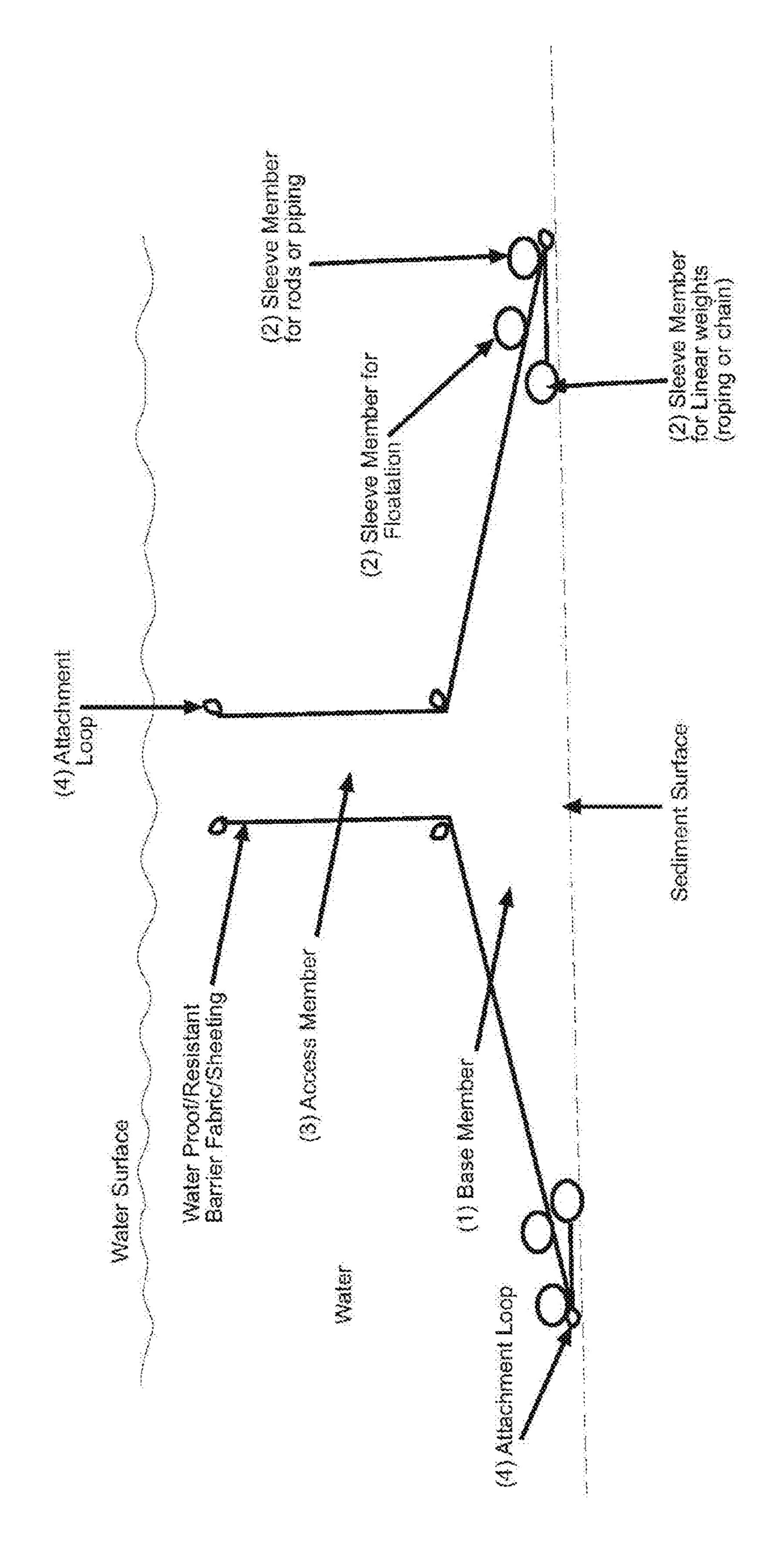
Vertical Slice of Cross-Section of Apparatus with two Access Members
