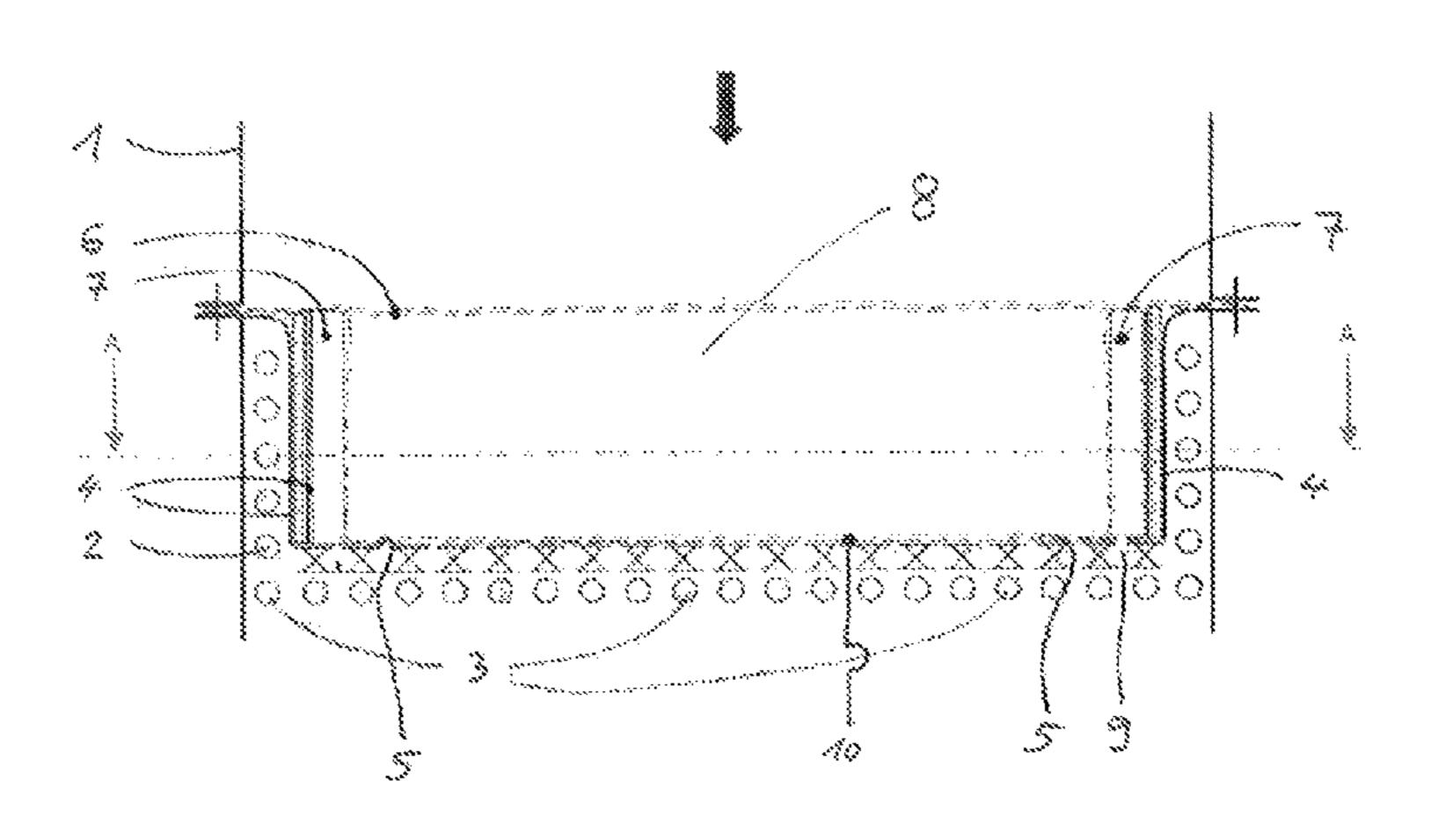
device D, the material for the thermal insulation layer S being selected from the group consisting of ceramic material, microporous material and silicate fibers.
