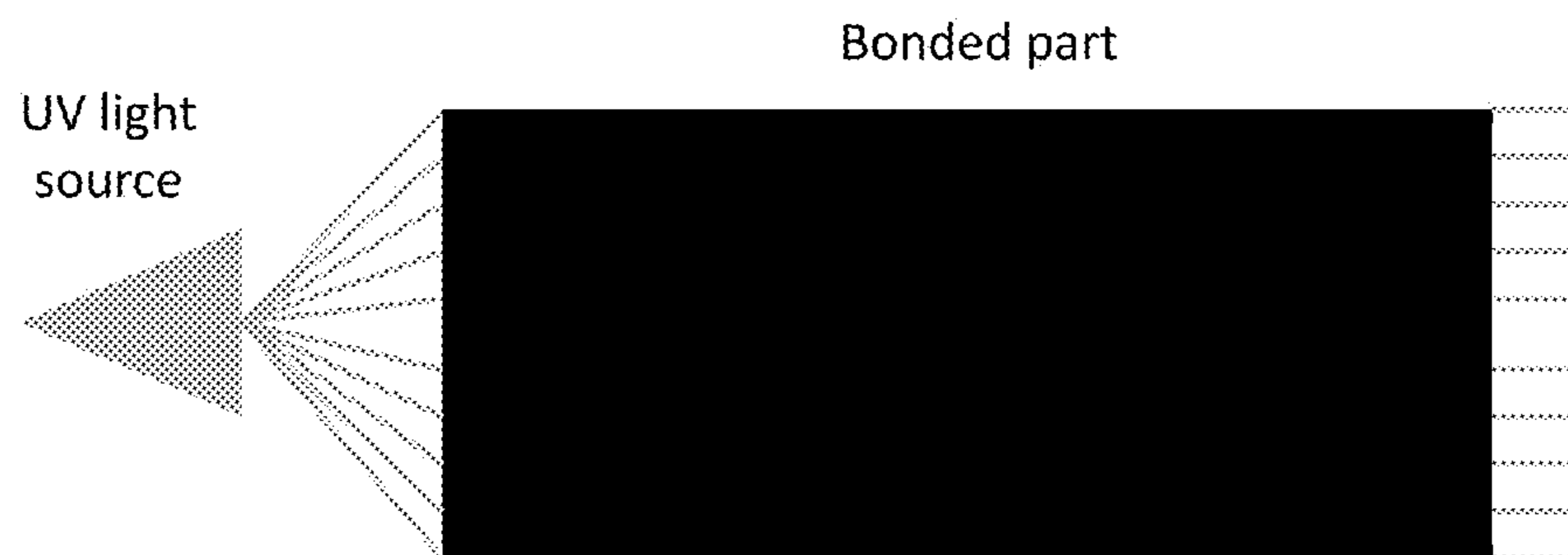
FIG 4. UV light source directed into the bond area inside the part
