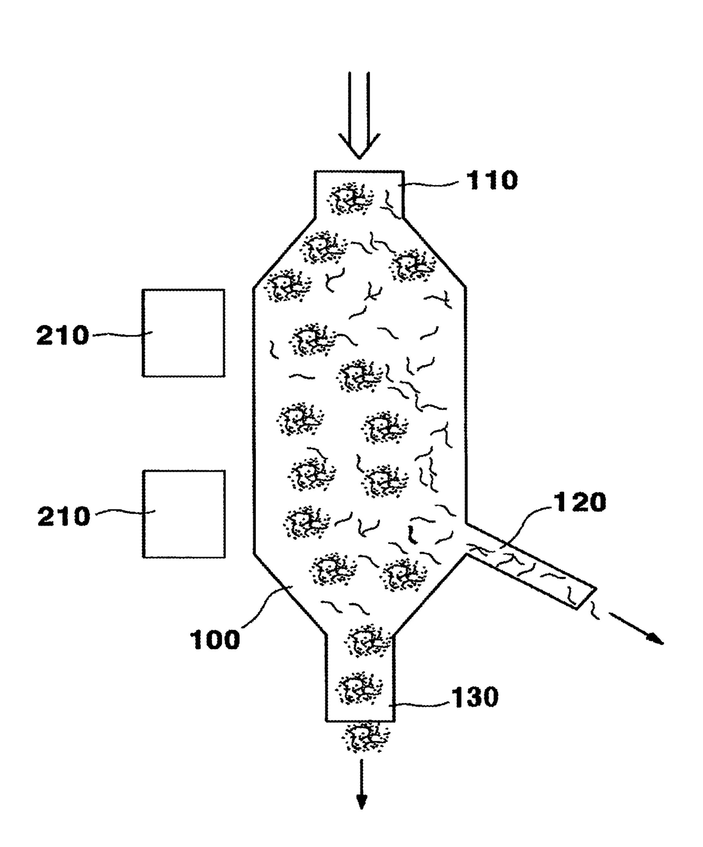
SIZE SEPARATING DEVICE FOR CARBON NANOTUBE AGGLOMERATE USING MAGNETIC FIELD, AND SEPARATING AND OBTAINING METHOD OF DISPERSED CARBON NANOTUBE USING THE SAME
