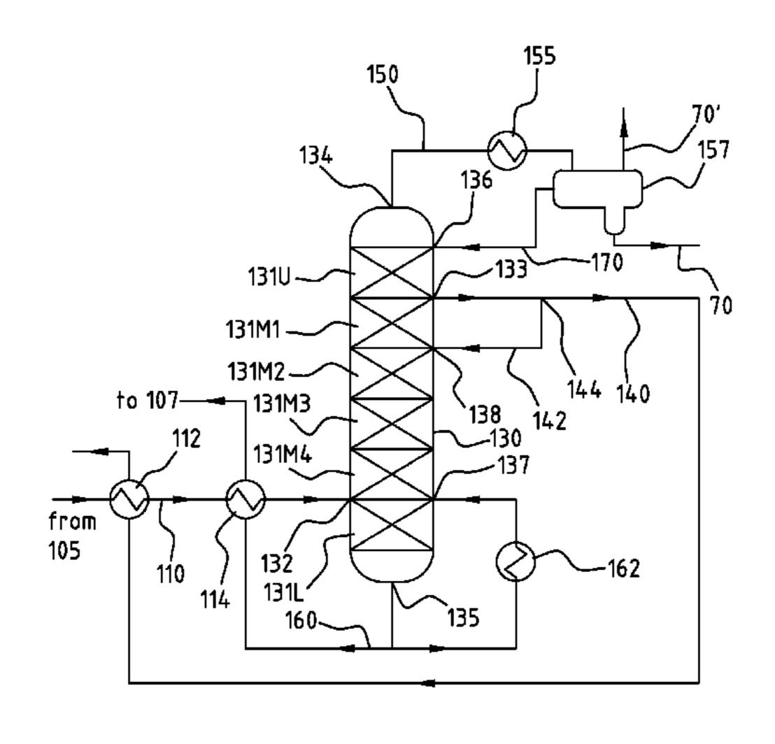
stage. A side stream of liquid water is drawn from the bottom of the upper theoretical stage in the distillation column.
