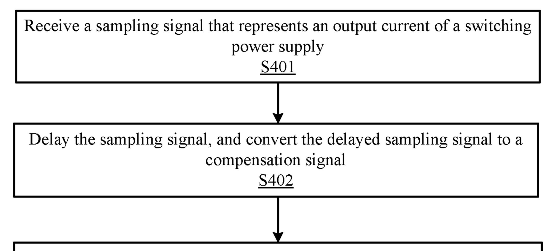
Regulate an output voltage of the switching power supply based on the compensation signal to compensate for a voltage loss generated by transmission of the output voltage to a load such that the load voltage is maintained as substantially consistent with an expected voltage at the load \$\frac{S403}{}\$
