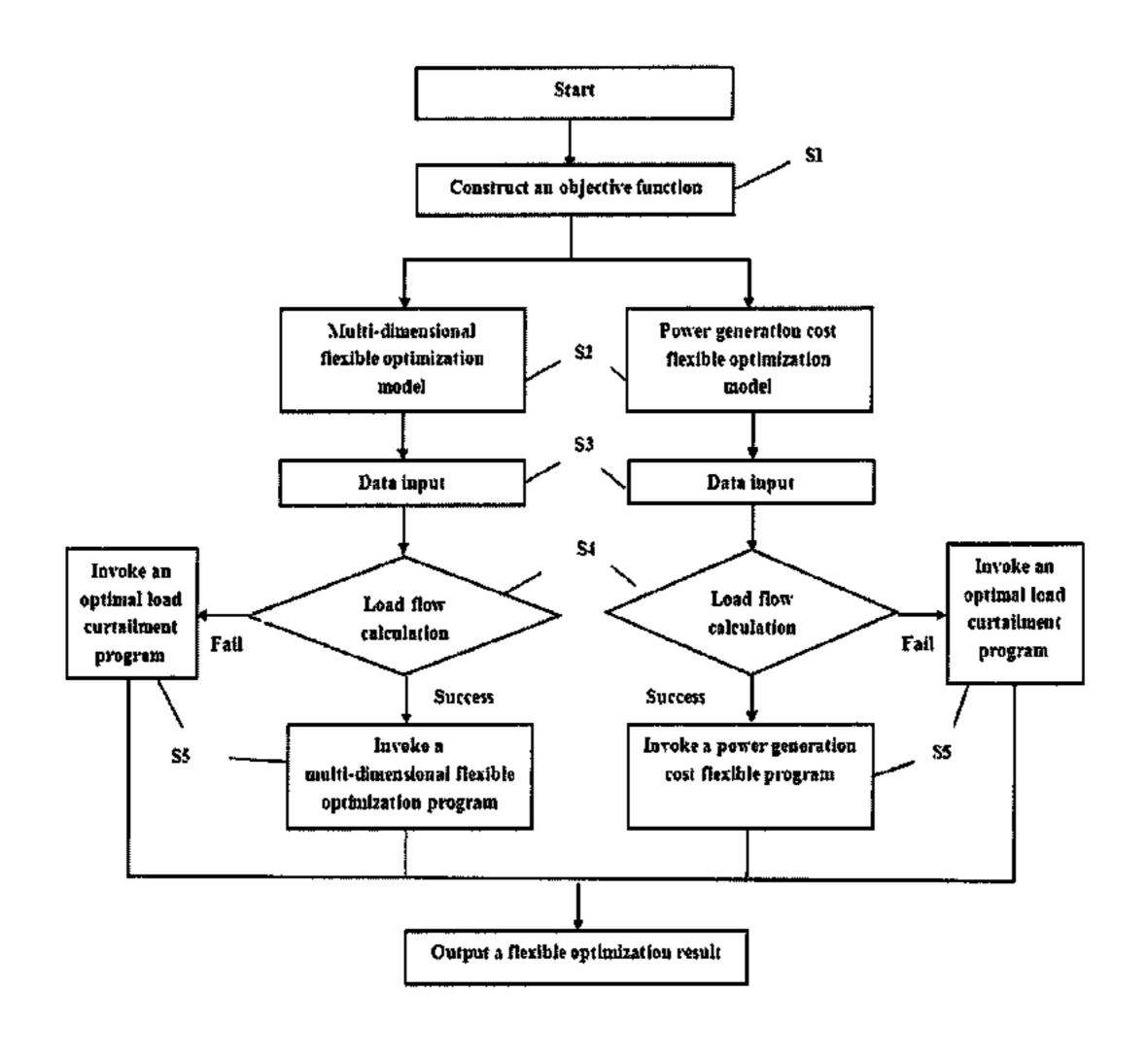
operating conditions of the electric power system, and a step S4 of carrying out load flow calculation.
