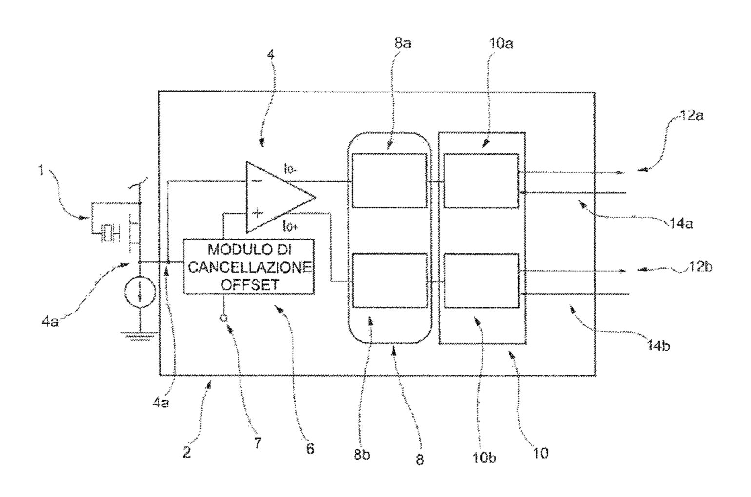
at least one neuron is adapted to receive said at least one current signal and to produce at least one output signal, said at least one output signal being a pulse train having a frequency proportional to said at least one current signal produced by the transconductance amplifier.
