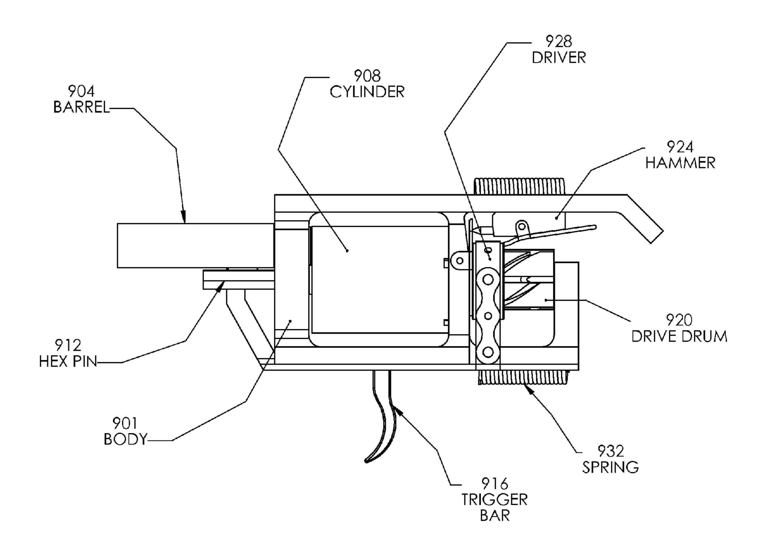
SIDE VIEW OF ACTION SAFE/AT REST POSITION
