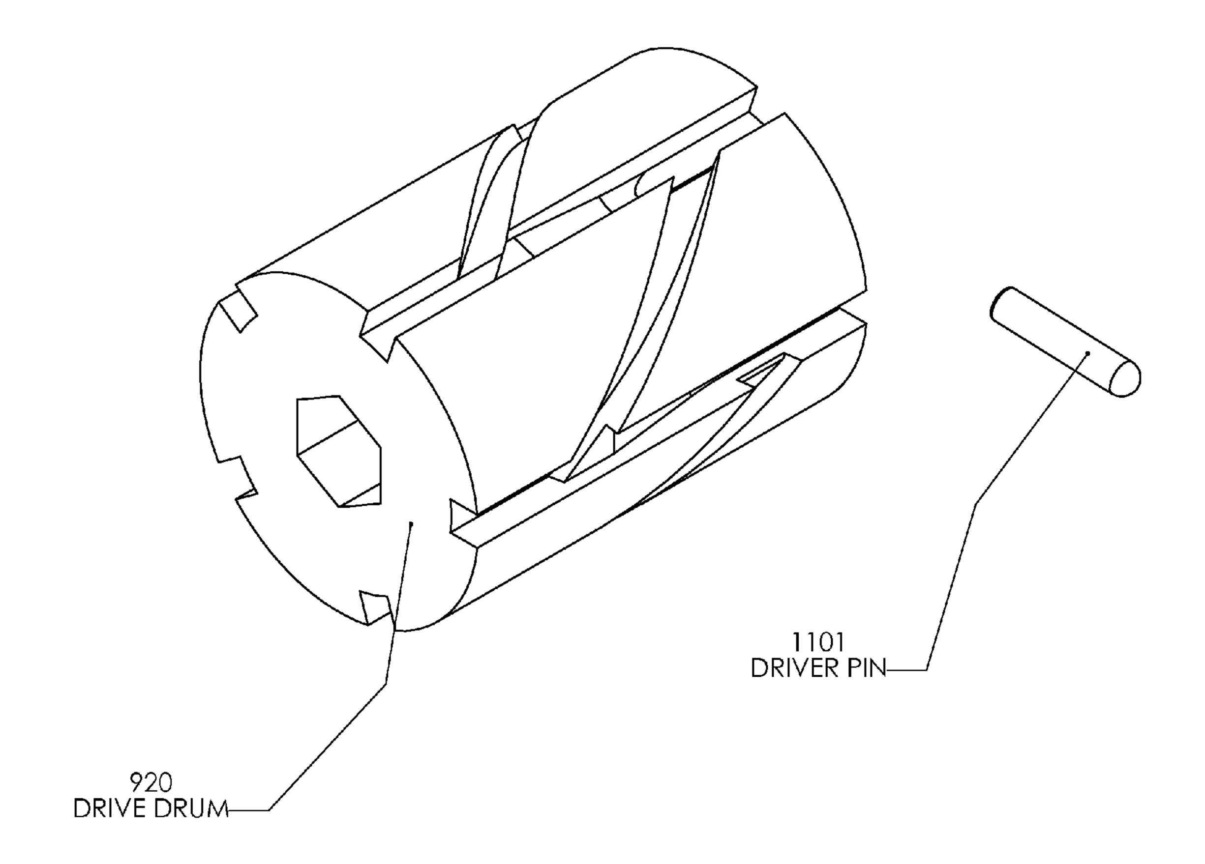
ISOMETRIC VIEW OF DRIVE DRUM 920 FIG 12
