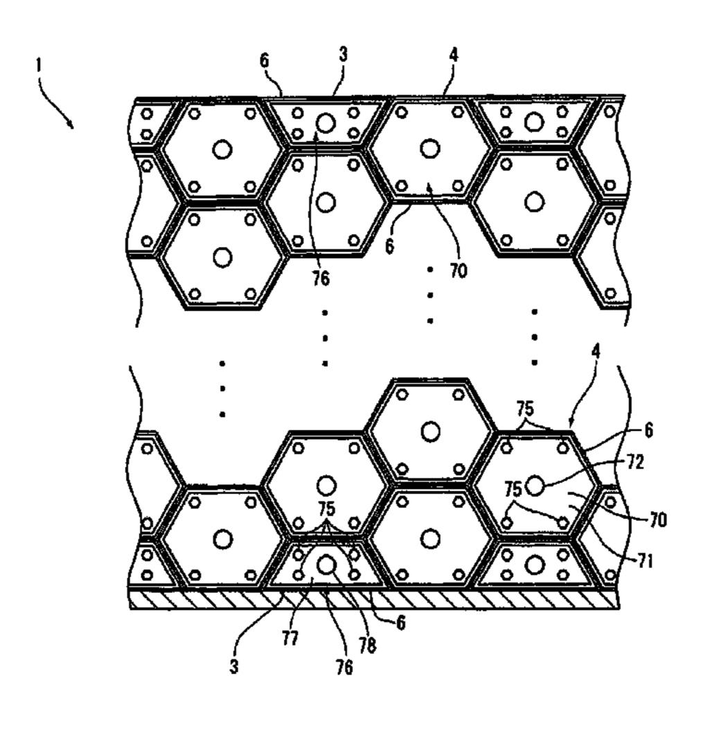
furnace; the refractory blocks are arranged such that each position of the hot-face end surface is positioned along the radial direction of the furnace at a predetermined reference position; and the refractory blocks are arrayed along the circumferential direction of an inside surface of the steel shell, thereby being stacked in a honeycomb manner.
