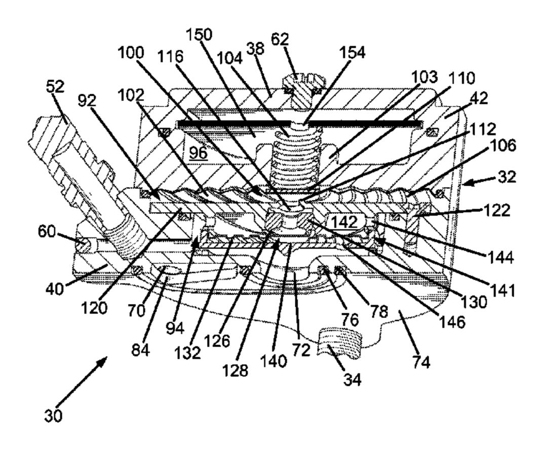
flow valve, and which deforms in response to a change in temperature in the valve assembly, thus negating temperature effects on the flow valve, allowing the flow valve to close at a consistent force across a range of operating temperatures.
