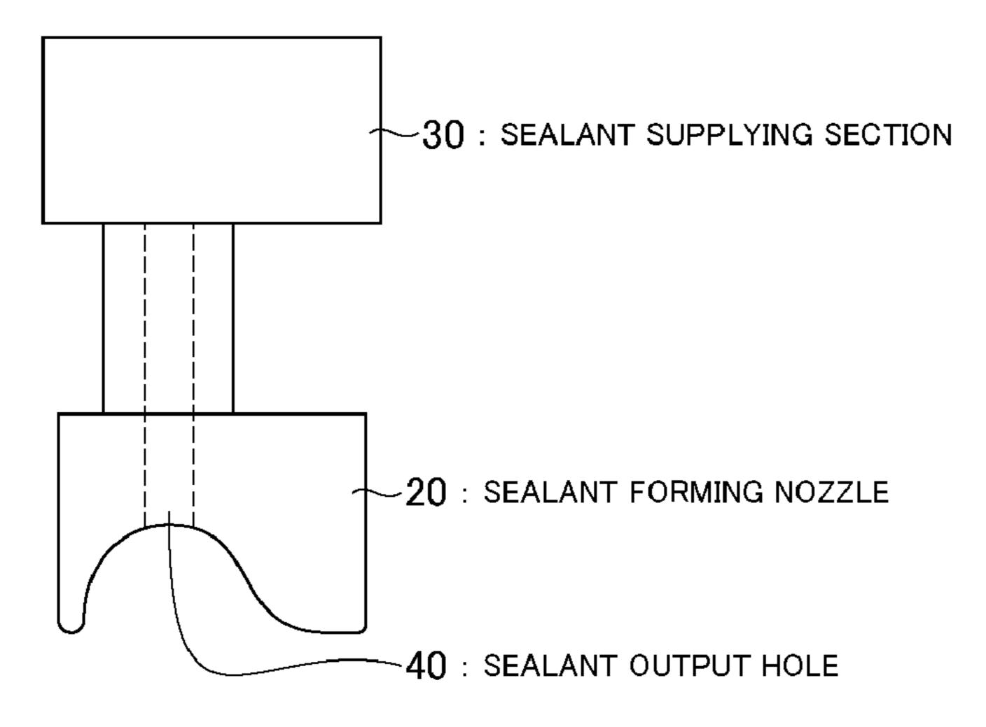
10 : SEALANT FORMING APPARATUS
