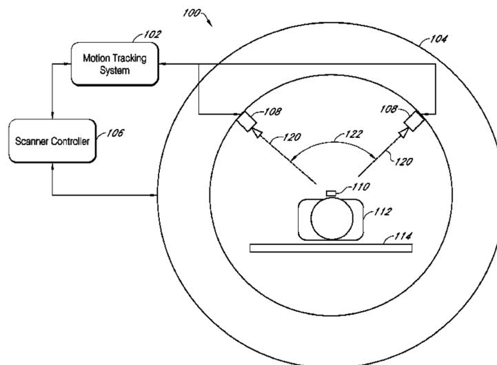
and a controller interface configured to generate tracking information based on the pose and to electronically transmit the tracking information to a scanner controller to enable compensation within a medical imaging scanner for object motion.
