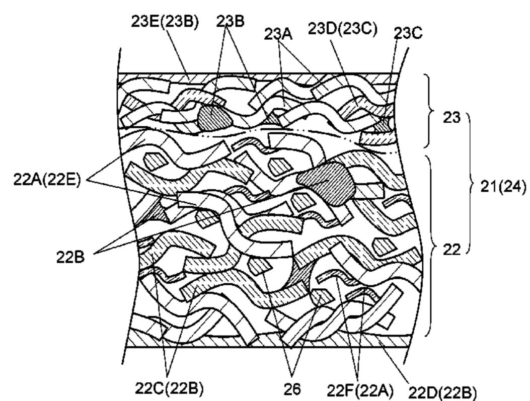
elastic modulus of 150 GPa or greater, and is formed by a papermaking process with the fibers.
