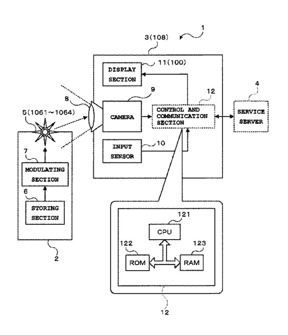
color change of the light emitting section emitting light by light emission control by the information transmitting device, from images consecutively captured by the camera, decodes the detected color change into information, and outputs the generated information to a display section.
