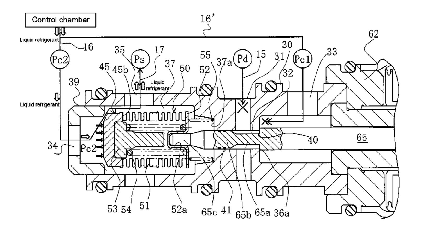
the valve, while contracting as the ambient pressure increases; and a solenoid that applies an electromagnetic drive force to control the main valve; wherein the pressuresensitive body is supported on one side by the driving rod of the solenoid in a manner permitting relative motion, while connected on the other side to the liquid-refrigerant discharge valve, wherein the discharge valve structure and discharge flow passages for discharging liquid refrigerant are simplified.
