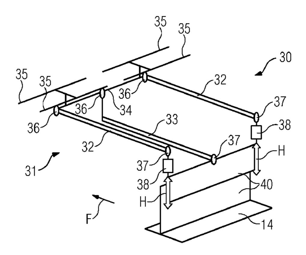
tors with an extended height range can be contacted without the current collector influencing the entire length of the vehicle.
