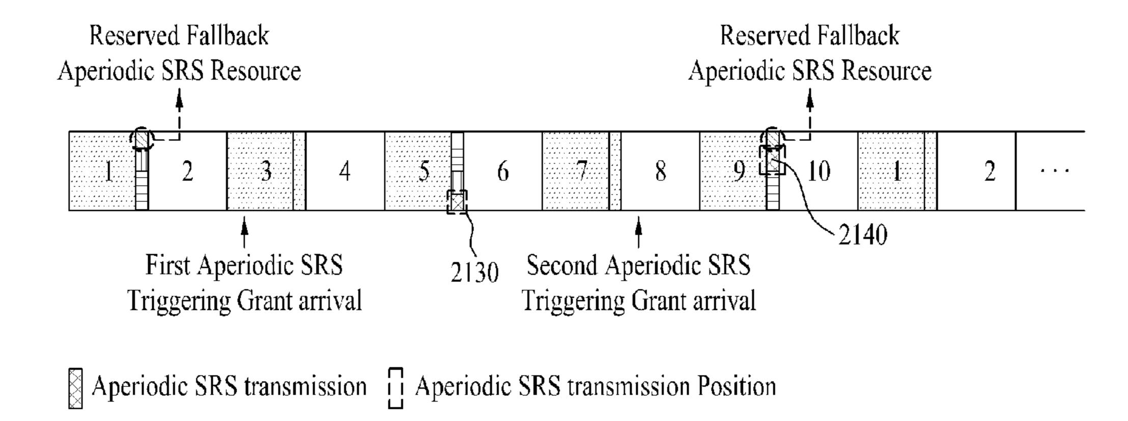
METHOD OF TERMINAL TRANSMITTING SOUNDING REFERENCE SIGNAL ON THE BASIS OF APERIODIC SOUNDING REFERENCE SIGNAL TRIGGERING AND METHOD FOR CONTROLLING UPLINK TRANSMISSION POWER TO TRANSMIT APERIODIC SOUNDING REFERENCE SIGNAL
