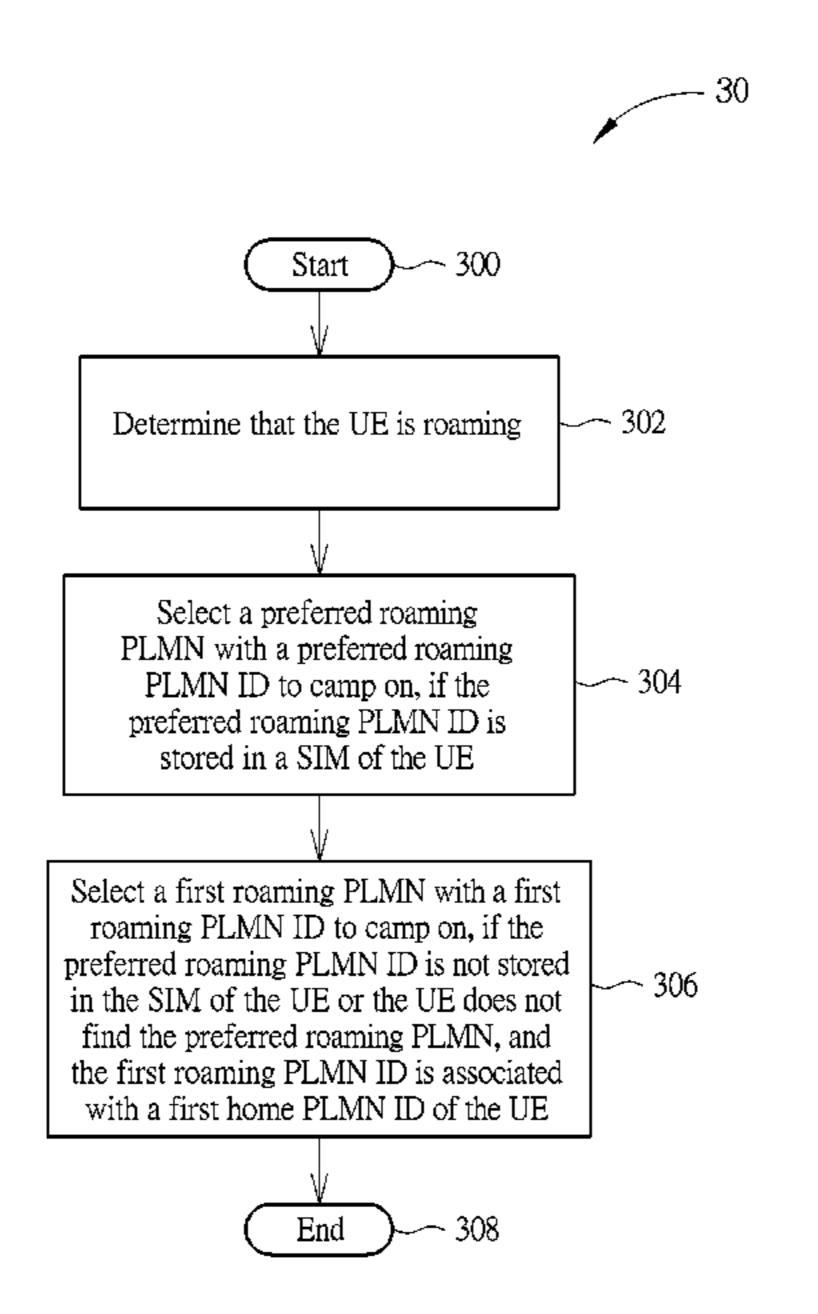
identity module (SIM) of the communication device; and selecting a first roaming PLMN with a first roaming PLMN ID to camp on, if the preferred roaming PLMN ID is not stored in the SIM of the communication device, or the communication device does not find the preferred roaming PLMN and the first roaming PLMN ID is associated with a first home PLMN ID of the communication device.
