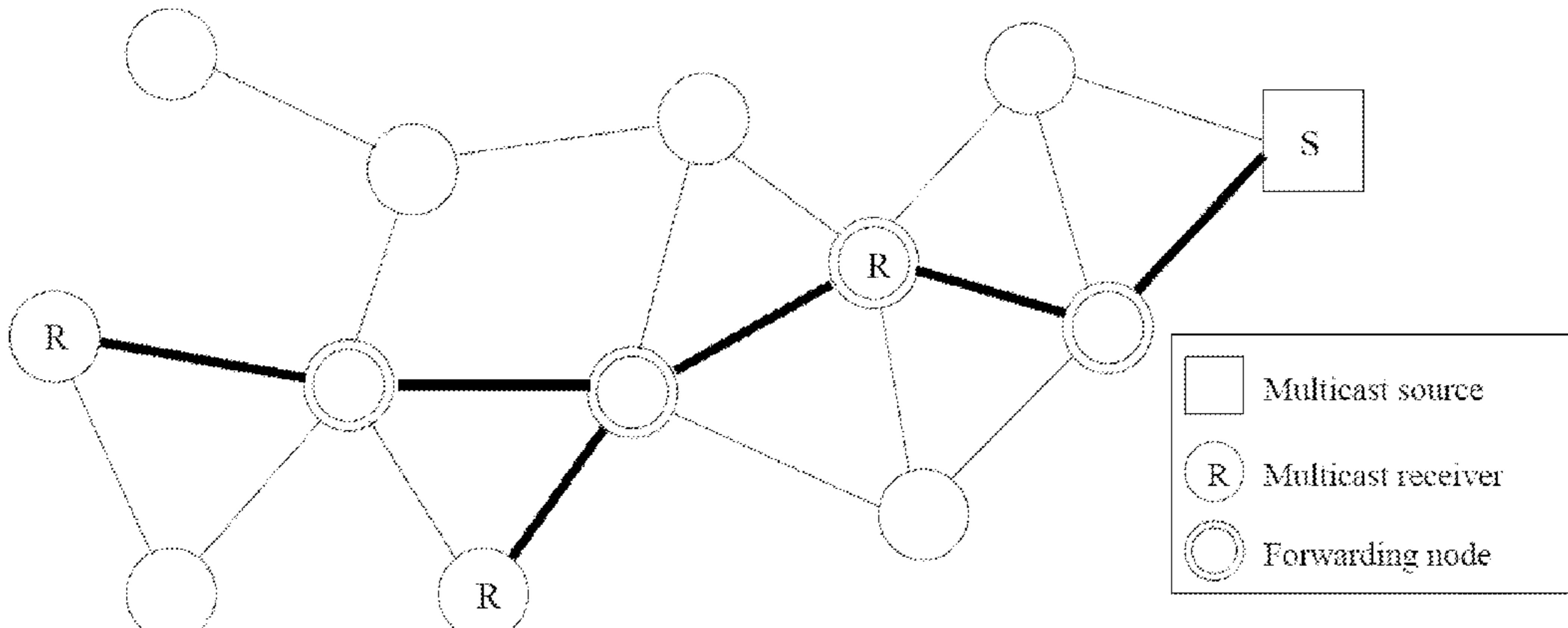
**Example of tree-based multicast forwarding structure**
