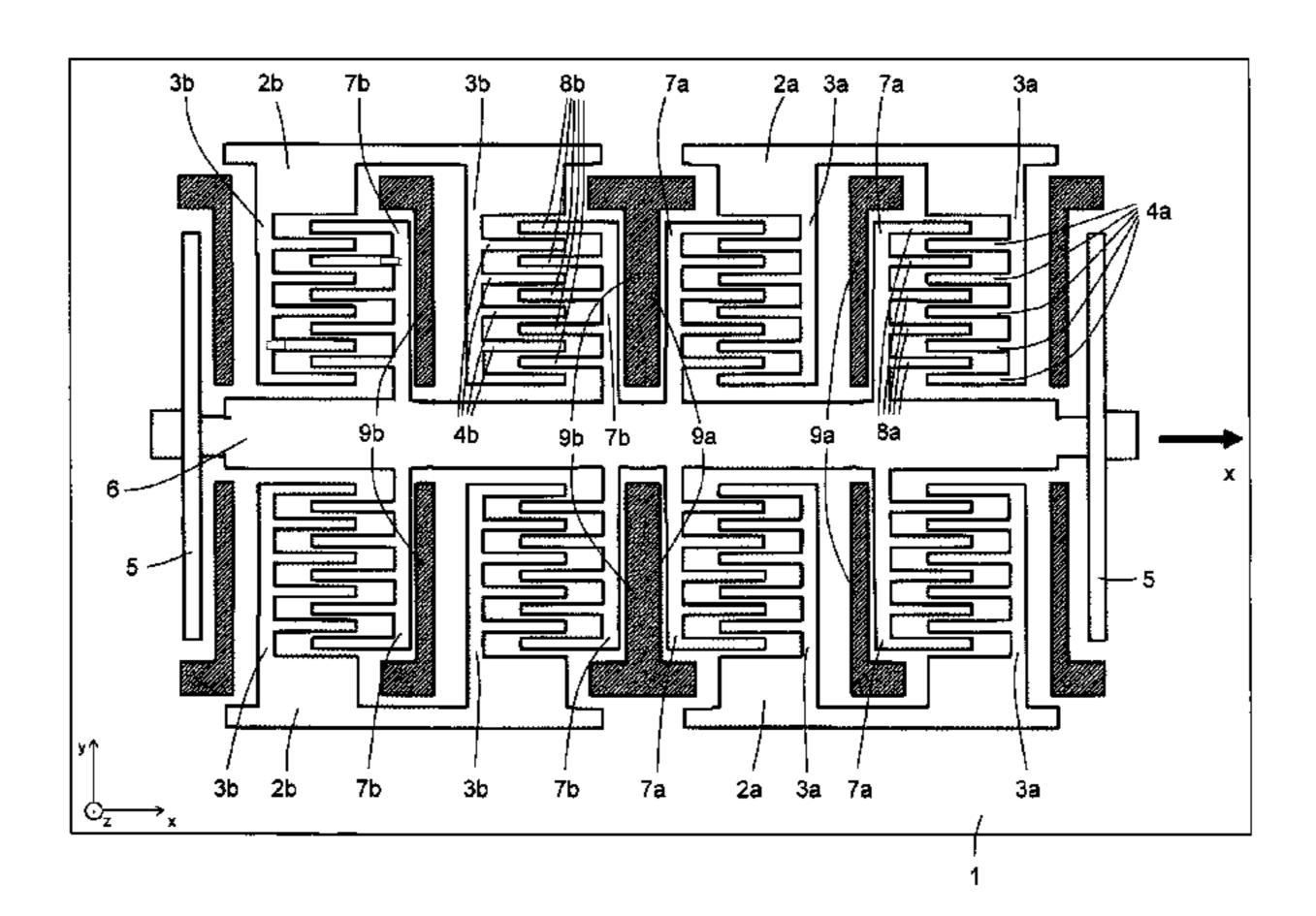
fixedly connected to the substrate and which is suitable for increasing a pneumatic damping of the sample mass during a deflection movement of the sample mass.
