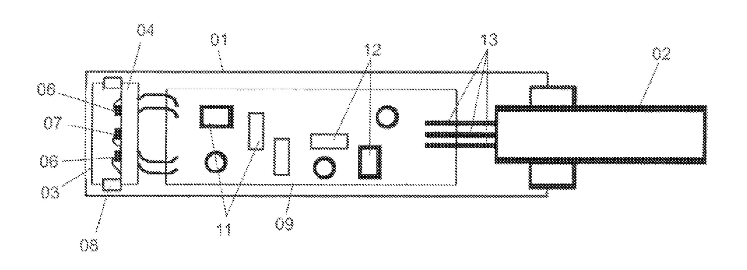
passes through the window are located in the sensor housing. Evaluating electronics arranged in the sensor housing are electrically connected at least to the receiver. The evaluating unit is designed to generate at least one digital sensor signal. The sensor unit further includes an electrical connection, which is led through the sensor housing and electrically connected to the evaluating electronics in the sensor housing.
