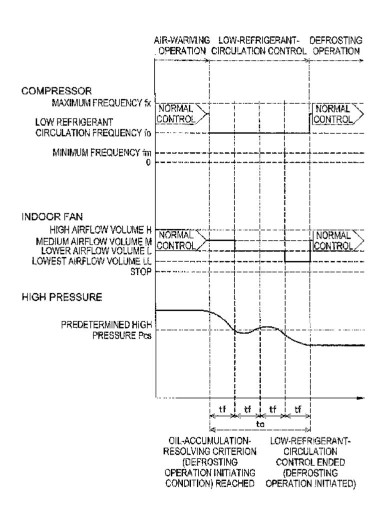
compressor, indoor heat exchanger, expansion valve, and outdoor heat exchanger in order, is performed for a predetermined time with an operating capacity of the compressor having been lowered to a predetermined capacity. The oil-accumulation resolving criterion is used to initiate an operation of defrosting the outdoor heat exchanger after the low-refrigerant-circulation control is performed.
