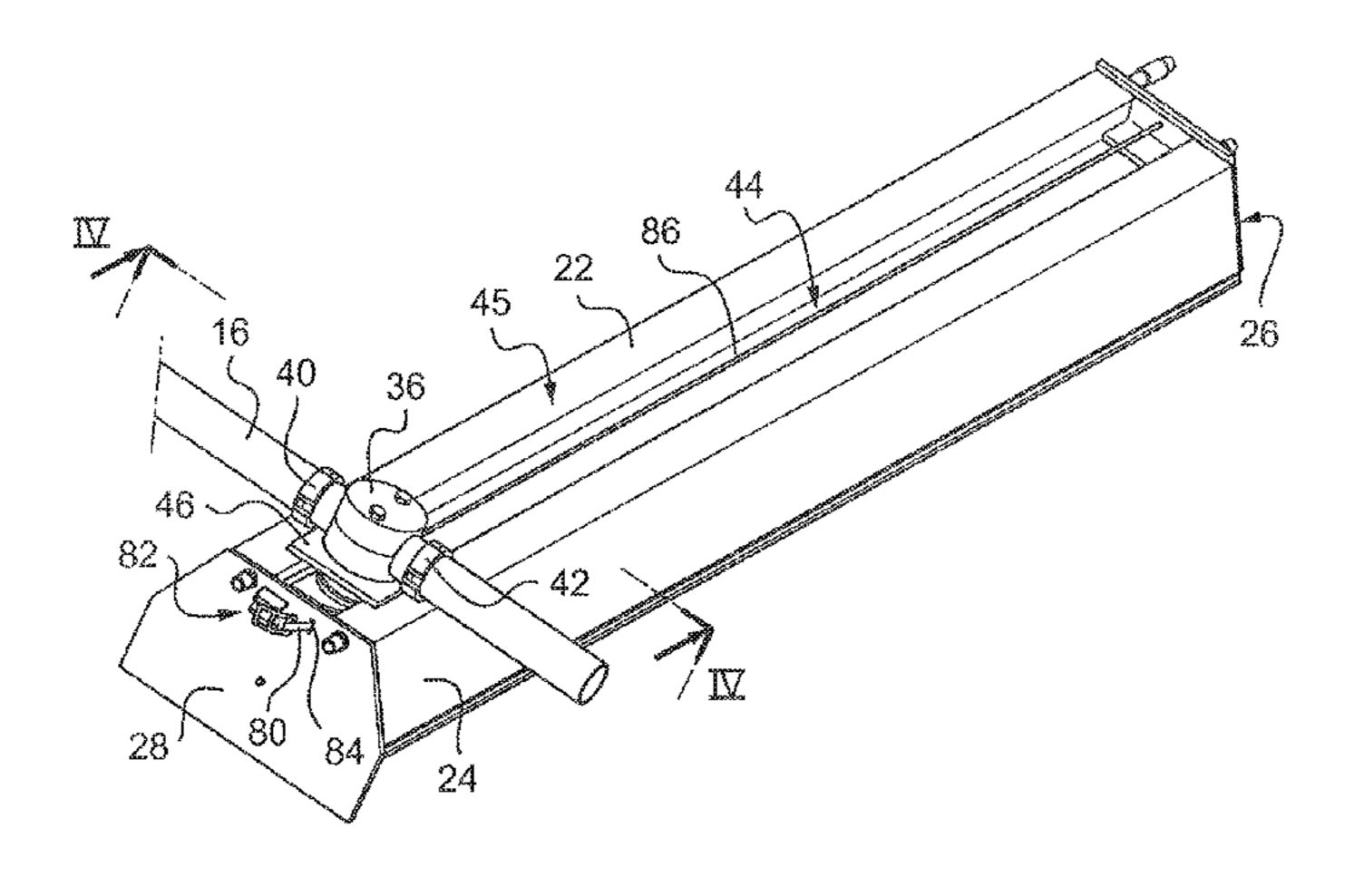
to install said longitudinal support (22) on the seabed (14) by deploying the section of rigid pipe (26) on the seabed (14).
