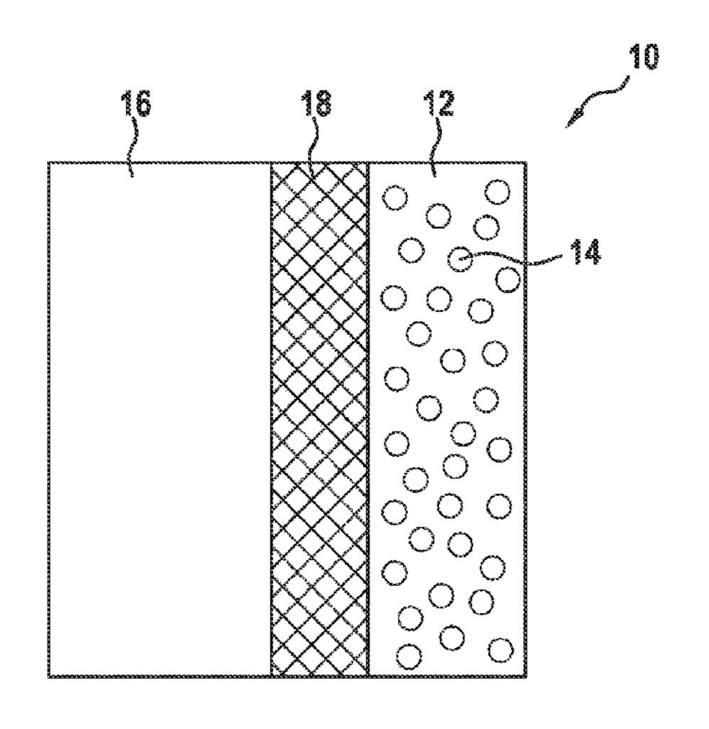
mixture of initial substances for formation of a lithium titanate; e) sintering the calcined product; and f) optionally removing the pore former from the calcined and optionally sintered product. Electrodes having a particularly defined pore structure can be generated with a method of this kind, thereby making possible particularly good capacity that is stable over the long term. A further subject is an electrode for use in a lithium-ion battery, as well as a lithium-ion battery.
