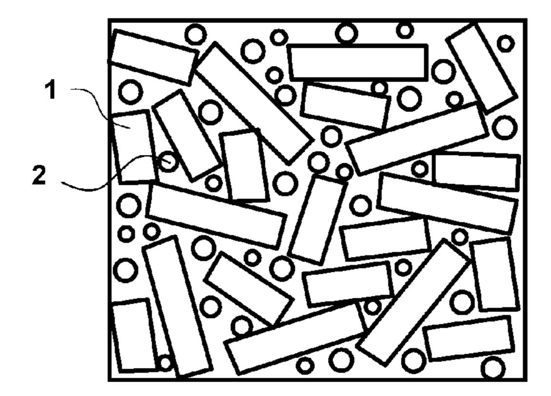
is dispersed among the pulverized powder of soft magnetic alloy ribbon. Further, it is characterized in that, preferably, the soft magnetic alloy ribbon is a Fe-based nano crystal alloy ribbon or a Fe-based alloy ribbon showing a Fe-based nano crystalline structure and that the pulverized powder has a nano crystalline structure.
