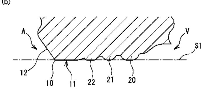
second annular projection starts slidable contact with the rotary shaft.
