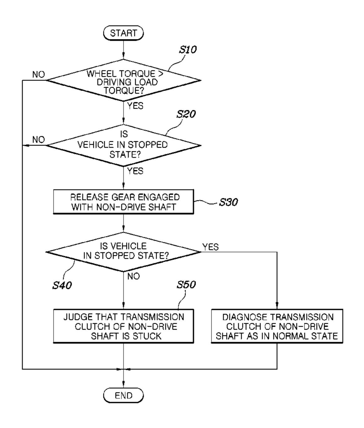
ing, by the controller, a gear engaged with a non-drive shaft, if, as a result of the confirming step, the vehicle is in a stopped state, reconfirming, by the controller, whether or not the vehicle is driving, after the releasing step, and judging, by the controller, that a transmission clutch of the non-drive shaft fails, if, as a result of the reconfirming step, the vehicle is driving.
