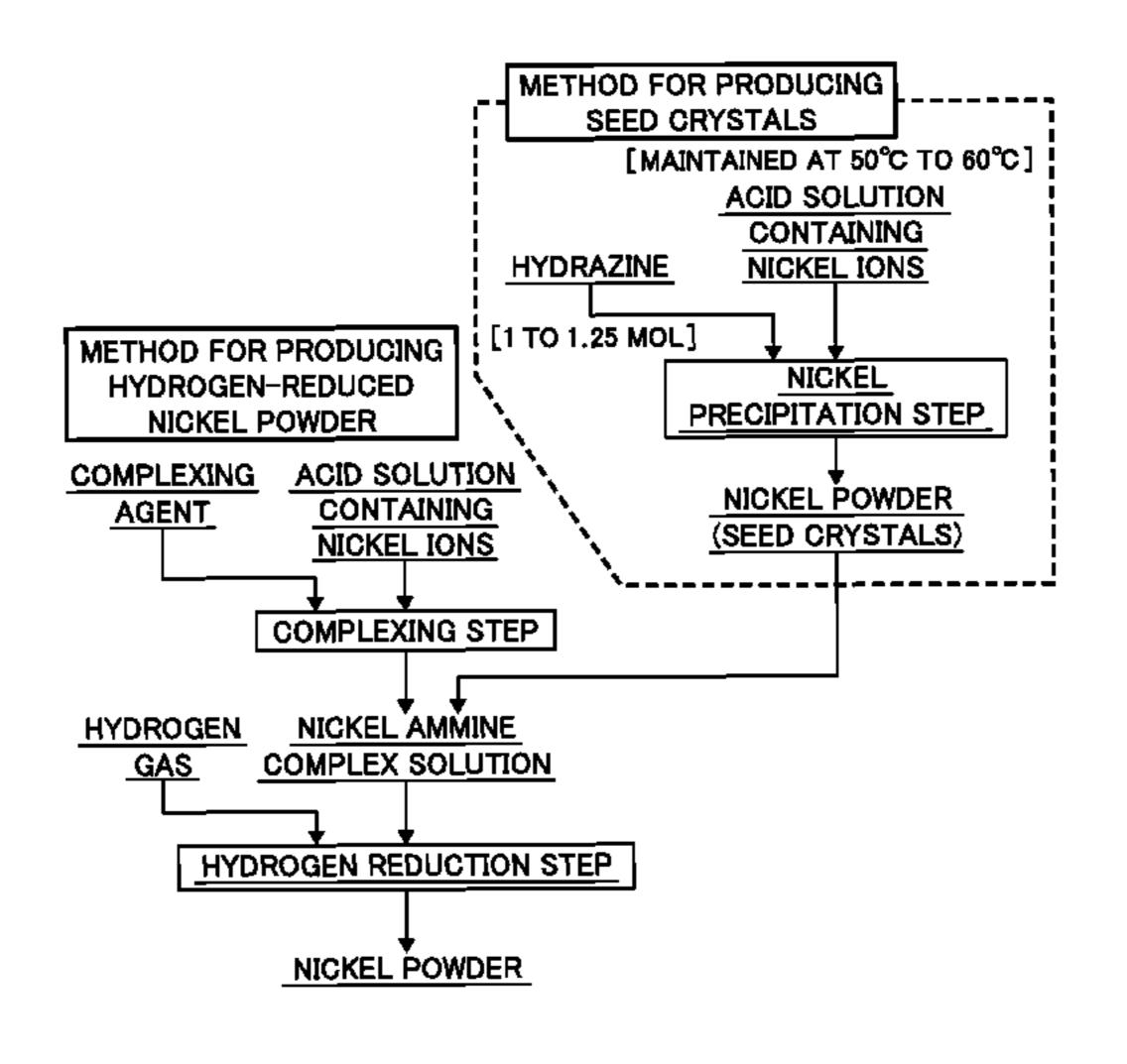
maintained at a temperature of 50 to 60° C., hydrazine of 1 to 1.25 mol per 1 mol of a nickel component contained in the acid solution to produce the seed crystals.
