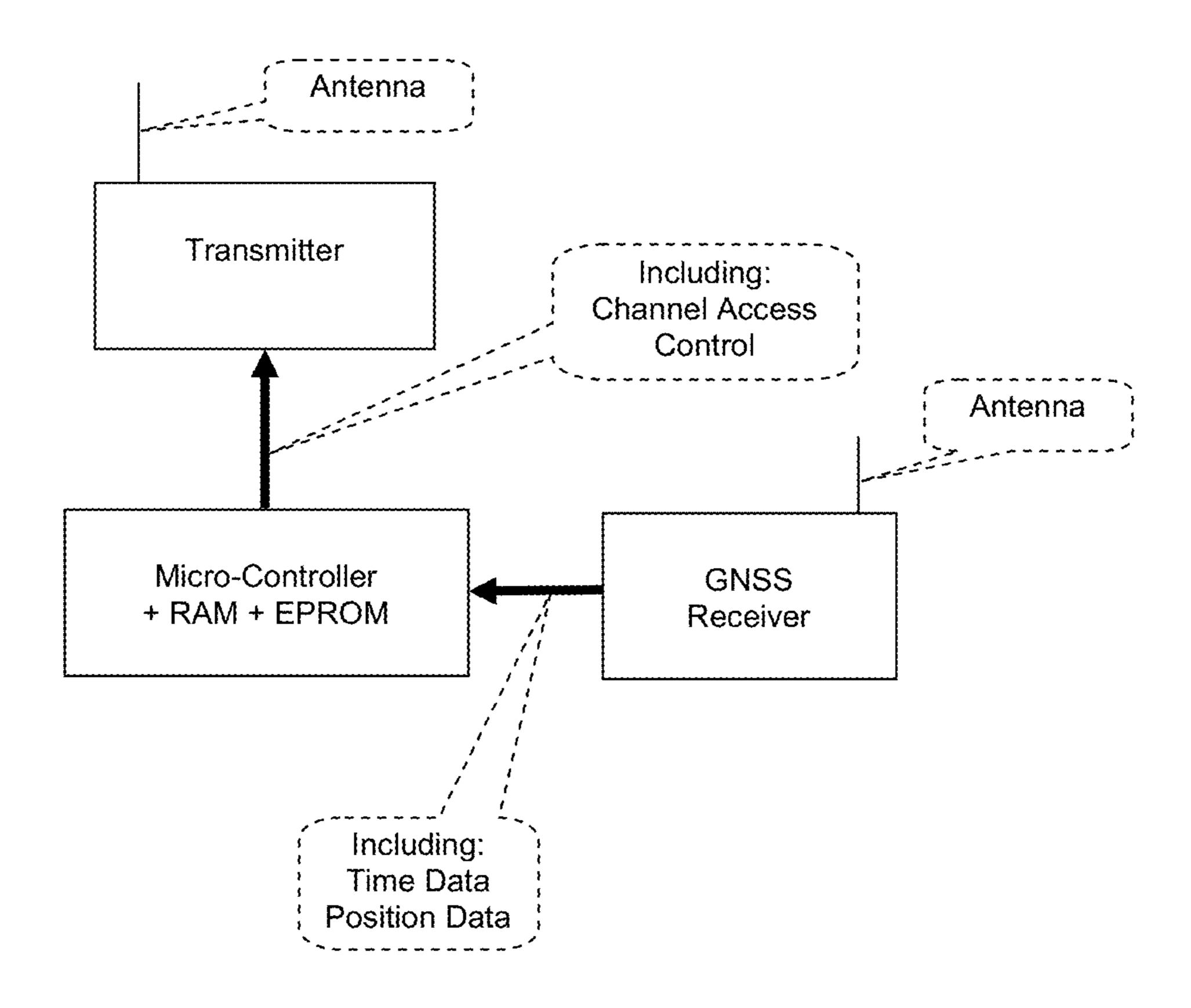
Fig. 5 – Receiver Block Diagram
