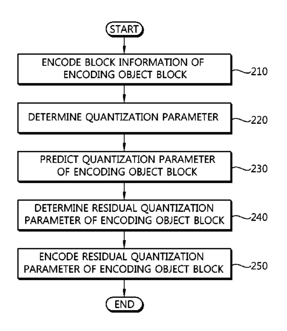
encoding and decoding apparatus which uses blocks having various sizes and depths as encoding and decoding units.
