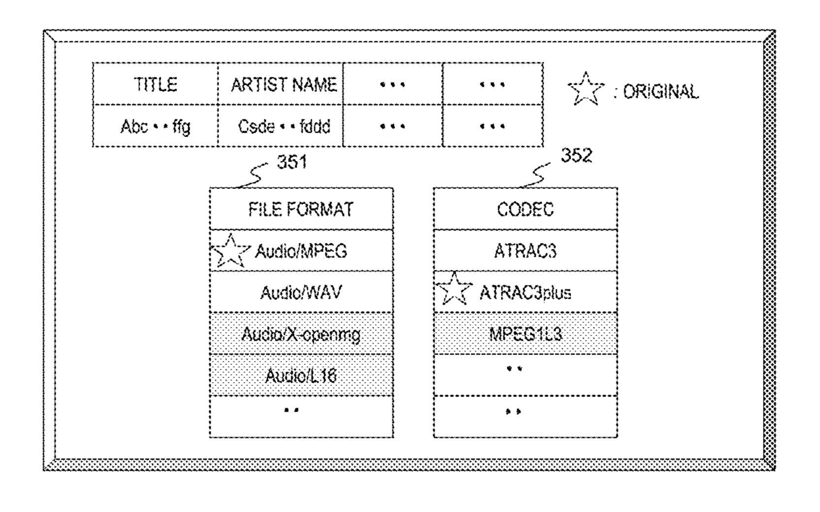
and is transmitted to the client. This structure allows the client to output a content transmission request in which the optimum data scheme is determined based on the data scheme of the original content. Therefore, high-quality data acquisition and playback can be achieved.
