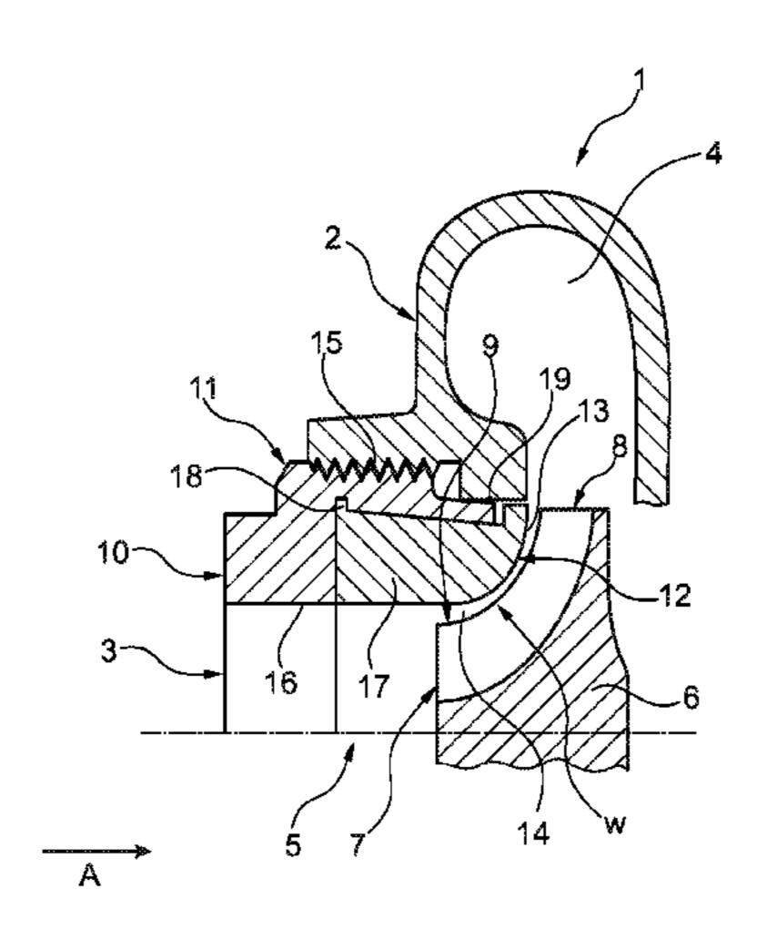
the fastening section (11) a gap width (w) of a passage gap (14) axially formed between the adapter element (10) and the compressor wheel (6) along the surface contours (9, 13) facing one another can be adjusted.
