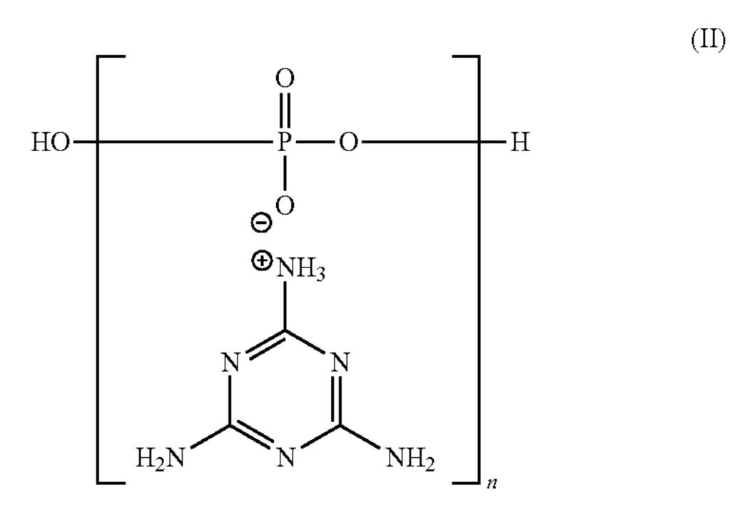
with  $n\geq 2$ , preferably ranging from 2 to 50. The melamine polyphosphate can be used in a quantity ranging from 0.01 to 3% by weight, calculated with respect to the polymer (a). Preferred melamine polyphosphate, according to the present invention, is characterized by a content of P<sub>2</sub>O<sub>5</sub> ranging from 31 to 35% by weight and a nitrogen content ranging from 40 to 44% by weight. This additive is present as a powder with an average particle-size ranging from 6 to 10 μm;
