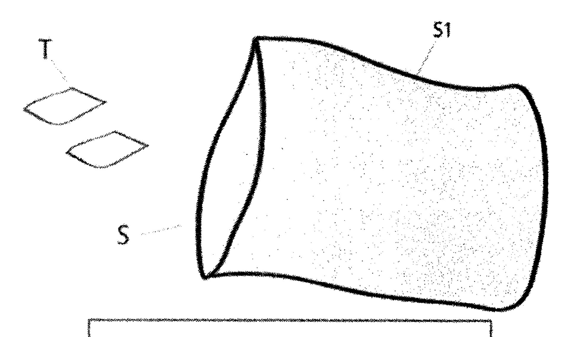
a) introduction of silk products or filaments into at least one very tightly-woven bag with high filtering capacity such as to allow the treatment liquid provided in phase b) to enter but not to allow the silk fibre to exit; said bag being bordered in such a way as to be sealed along the perimeter in correspondence of the seams;
