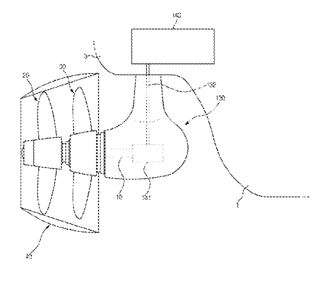
which extends from to the lower part of the hull, and which is installed so as to envelope the counter rotation device and the motor.
