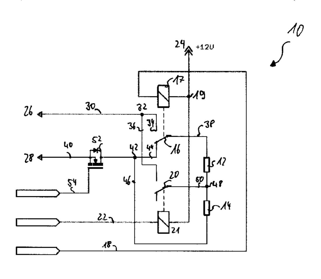
second heating mode in which the first resistance heating device and the second resistance heating device are electrically connected in parallel. A vehicle having electric heating as well as to a method for controlling electric heating is also provided.
