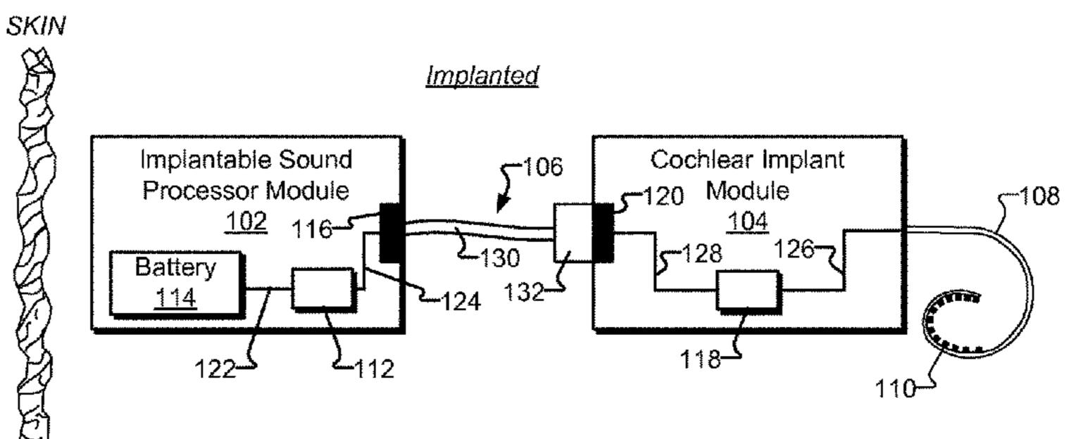
optical transmission of the data and/or the power from the sound processor circuitry to the cochlear implant circuitry while the implantable sound processor module is removably coupled to the cochlear implant module by way of the optical connector assembly.
