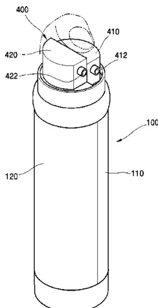
(410) and the second pressing cap (420) are combined and disposed on the top of the container (100) to be vertically movable, a rail (414) is vertically and convexly formed on a coupling side of the first pressing cap (410), and a rail groove (424) where the rail (414) is inserted is vertically and concavely formed on a coupling side of the second pressing cap (420), so the first pressing cap (410) and the second pressing cap (420) independently move.
